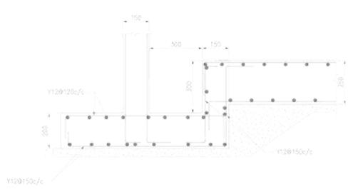
TYP. REINF. DETAIL FOR SUMP
